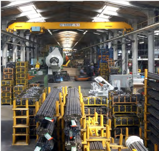
The 40mm steel bars used for the boules. The machine in the background (1 of 6) is used to create the outer casings.
